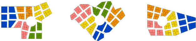
Fig. 15. Design of atrium. Here shows the commercial space layouts generated with an atrium, which is incorporated as a constraint in the generation.
